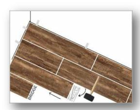
Step 7: Place wood block at end of plank and tap with hammer to lock ends of planks together.
