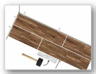
Step 5: THIS IS AN IMPORTANT STEP! Use a rubber mallet or hammer and a wood block. Tap the block to tap long edge of the plank to ensure a tight fit. MAKE SURE THERE IS NO GAPPING AS IT CAN COMPROMISE THE LOCKING SYSTEM!
