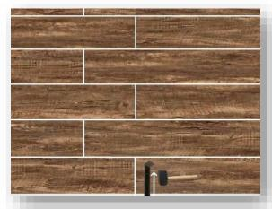
**Step 9**: Use a hammer and pull bar to lock long edges of planks on the final row.
