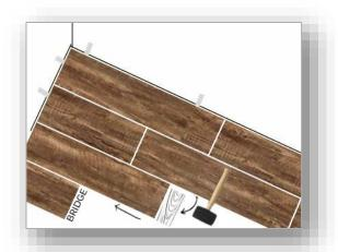
Step 7: Place wood block at end of plank and tap with hammer to lock ends of planks together.
