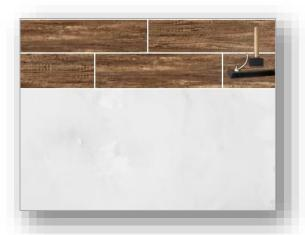
**Step 8**: Use a hammer and pull bar to lock the final piece in the row. Insert a spacer at end of the row. Continue installation on next row until final row.
